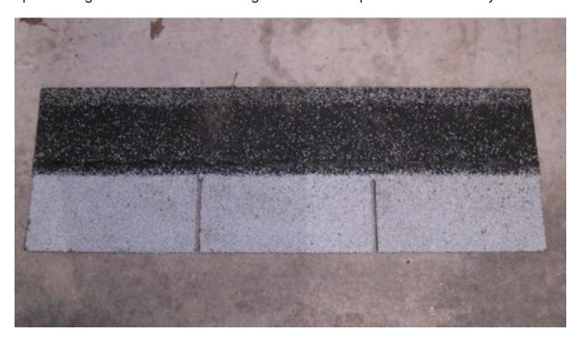
The photo above is a standard three-tab shingle. Each white tab is just under 12-inches wide and the tabs are 5-inches high. The wider black strip above the tabs will be covered by the next row of shingles. If you use these shingles on a roof, all you'll see are the white tabs once all the shingles are installed.
